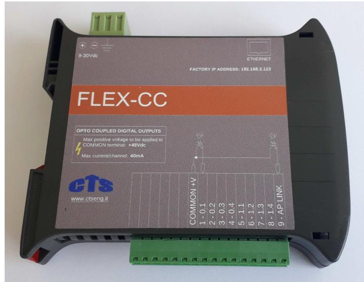
FLEX-CC provides 8 + 1 digital outputs, whose status is displayed by LEDs on the front panel of the card. Outputs 1...8 are user configurable via Traffic Dot. Output 9 is not configurable and represent the FLEX-CC / AP link status: led off means disconnected link, led on means connected link.
